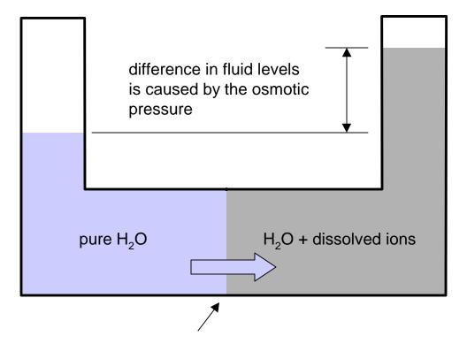
Semipermeable membrane allows water to pass, but not dissolved ions.
